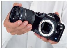
The image sensor is put at risk through dust entering during lens changes.
